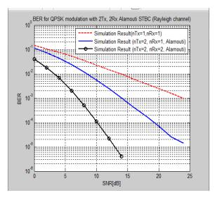
Fig8: BER for QPSK Modulation with 2x2 Alamouti STBC
