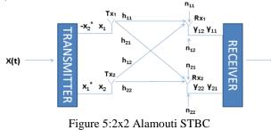
The 2x2 Alamouti STBC System is shown in figure 5 which is similar to 2x1 Alamouti but we have one more receiver antenna. This system is consists of 2 Transmitter and 2 Receiver. Working principle is also similar to 2x1 Alamouti. In 2x1 Alamouti we send block codes to just one receiver but in this system we send block codes to 2 receiver.
