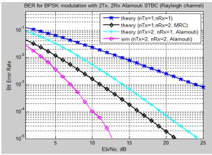
Fig7: BER for BPSK modulation for 2x2 Alamouti STBC
